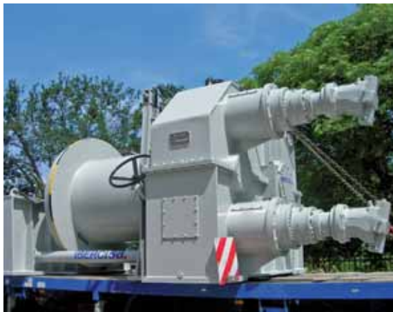
Auxiliary Anchor Winch Vessel: Charles Darwin/Owner: Jan de Nul/Country: Belgium
