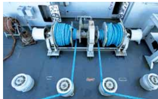
Mooring winch 2x220 m Ø96 mm rope
