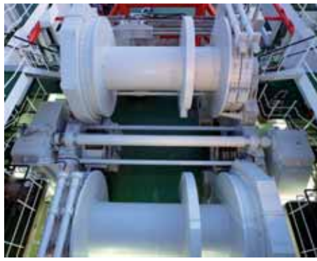
Anchor Handling Towing Winch 350 Tons Electrically Driven Vessel: Bylgia Owner: Heerema Marine Contractors Country: Netherland
