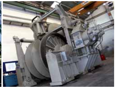
Waterfall Type Towing Winch 2x1000 m ø64 mm
