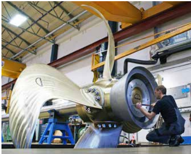
MAN Alpha Kappel propeller – four-bladed CP with fairing cone for rudder bulb
