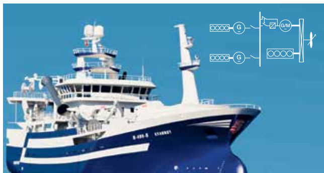
HyProp ECO: Hybrid propulsion system
