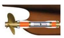
Our Water Quality Package is a self-contained pumping unit which removes abrasive solids from the water supply (down to 40-50 microns). As water enters the forward seal, it flows through the COMPAC bearings and exits at the stern. Flow rate is monitored by low flow alarms.
