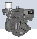
4-cylinder, 4-stroke, direct-injected, turbocharged aftercooled (TA version) marine diesel engine. Bore x Stroke (mm): 108 x 130 Displacement (I): 4.76
