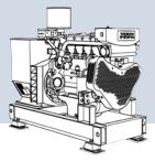
4-cylinder, 4-stroke, direct-injected, turbocharged marine diesel engine.
