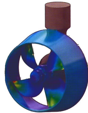
Hydrodynamic optimization by CFD simulations
