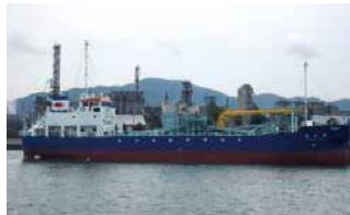
Tokuyama Maru, cement tanker, Tokuyama Kairiku Unso K.K. 6DEM-23L × 1, Yamanaka Shipbuilding Co., Ltd.
