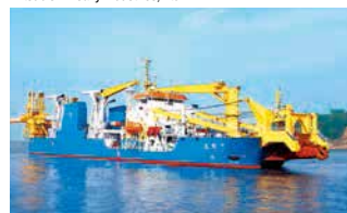
Tianjing Hao, 4,500 m³ self-propelling dredger, Tianjing Waterway Bureau 8DKM-36(L) × 2, pump-driving 8DK-36 × 2
