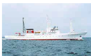
Ikitsuki, fishery control boat, K.K. Taishu 8DKM-28L × 1, Izutsu Shipyard Co., Ltd.
