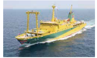
Tachibana Maru, ferry, Tokai Kisen Co., Ltd. 6DE-23 × 3, Shimonoeki Shipyard & Machinery Works, Mitsubishi Heavy Industries, Ltd.
