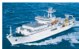
Subaru, cable laying ship (electric propulsion), Nippon Telegraph & Telephone Corp. 8DK-32 × 4, Shimonoseki Shipyard & Machinery Works, Mitsubishi Heavy Industries, Ltd.
