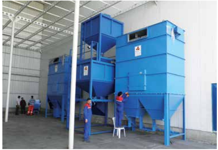
Our 50.000m 3 /h Dust Collectors for Shipyard
