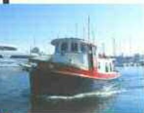
The **style** of the hull is traditional elliptical stern tug above the waterline combined with a trawler-yacht underbody of much lighter displacement than would be found on a working tug. The superstructure is a blend of a traditional tug pilothouse with a deckhouse needed for the accommodation.
