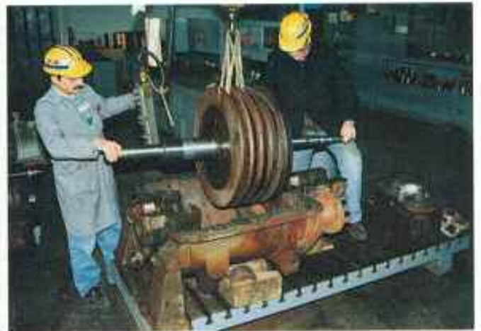
Overhauling of a steam turbine.
