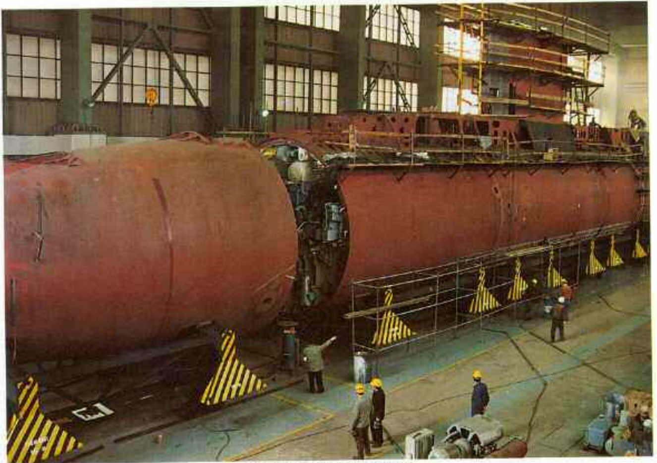
Bringing the main sections together
