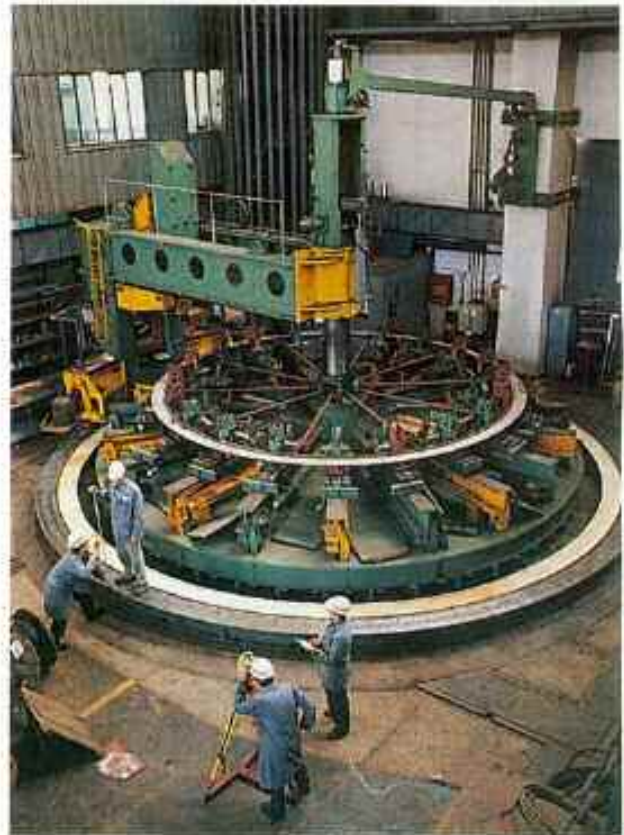
Tack weld Bevel-Jig is a comprehensive tool for the machining of frames, frame segments and transition rings for submarine construction. It can processes materials with a diameter of 3100 mm to 7500 mm and thickness up to 800 mm.
