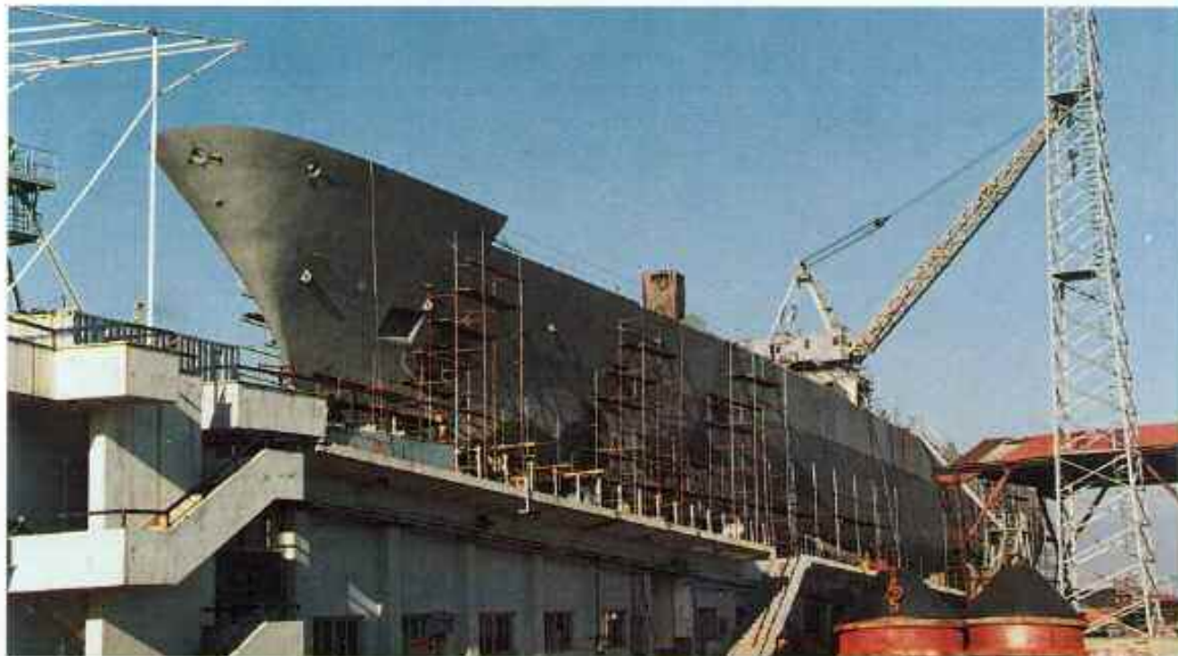
Hull construction on the slip-way
