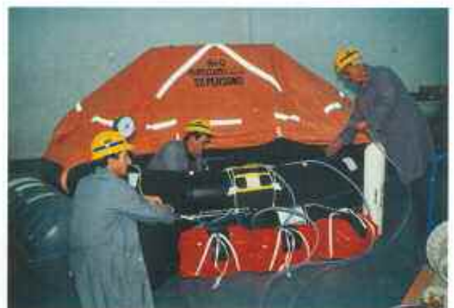
In the life-raft-repairing workshop, 20 different types of life rafts in the Turkish Navy are tested and certified.
