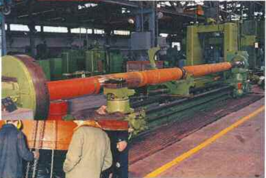
Machining of a propeller shaft.
