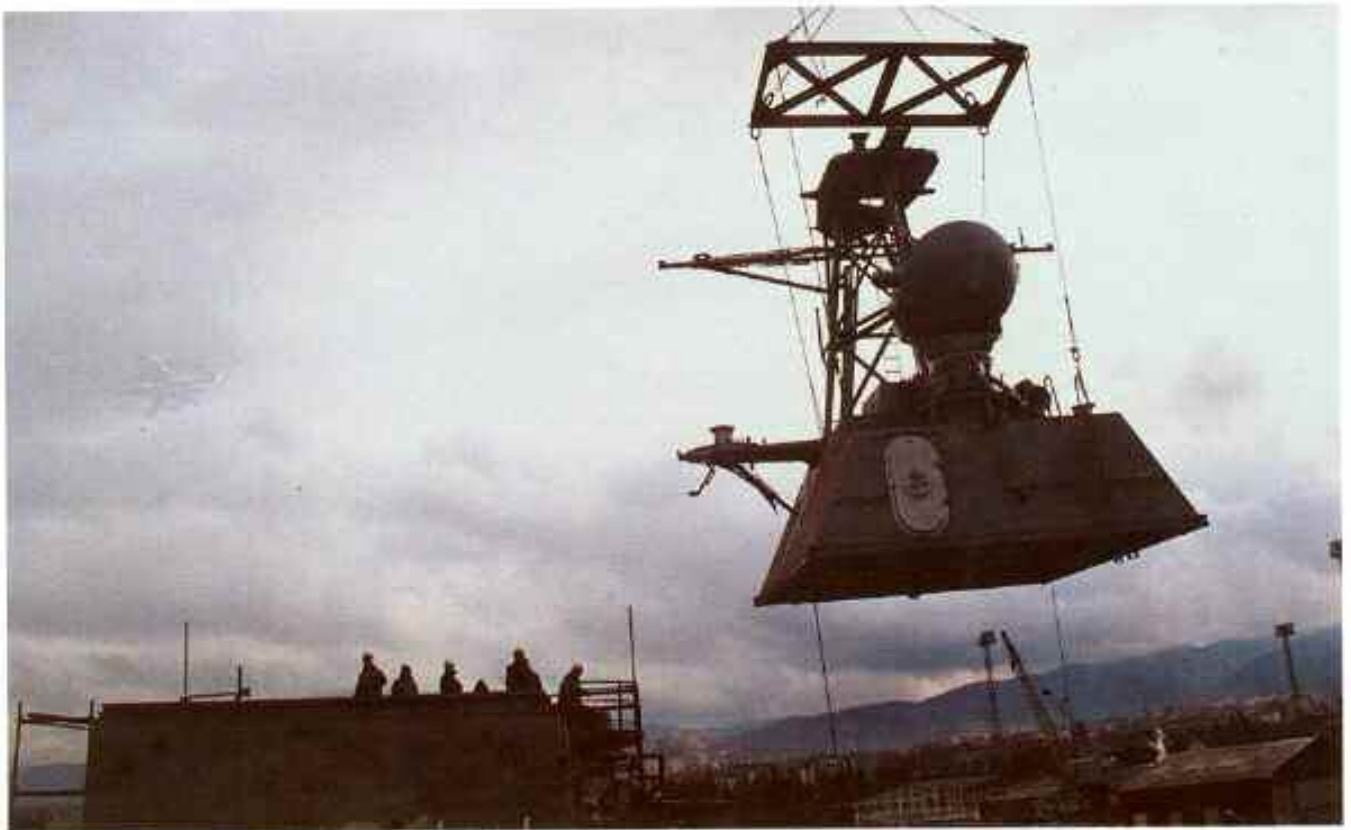
Transferring the fire control radar on board
