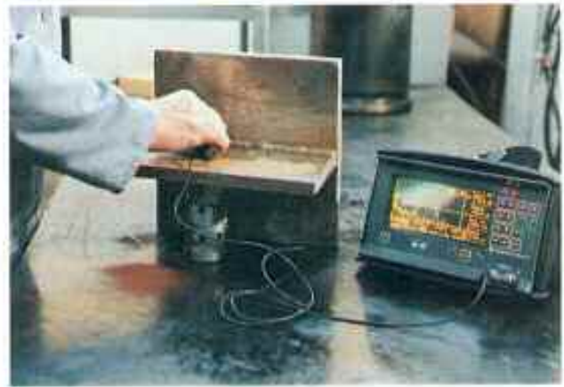
With non-destructive inspection methods not only the welding performed, but also the welders themselves are certified.
