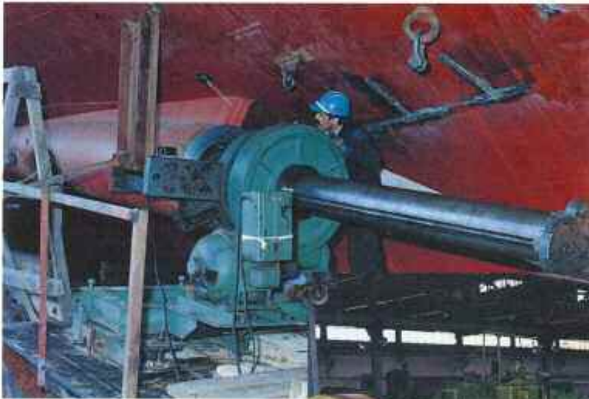
Shaft boring of a new construction.
