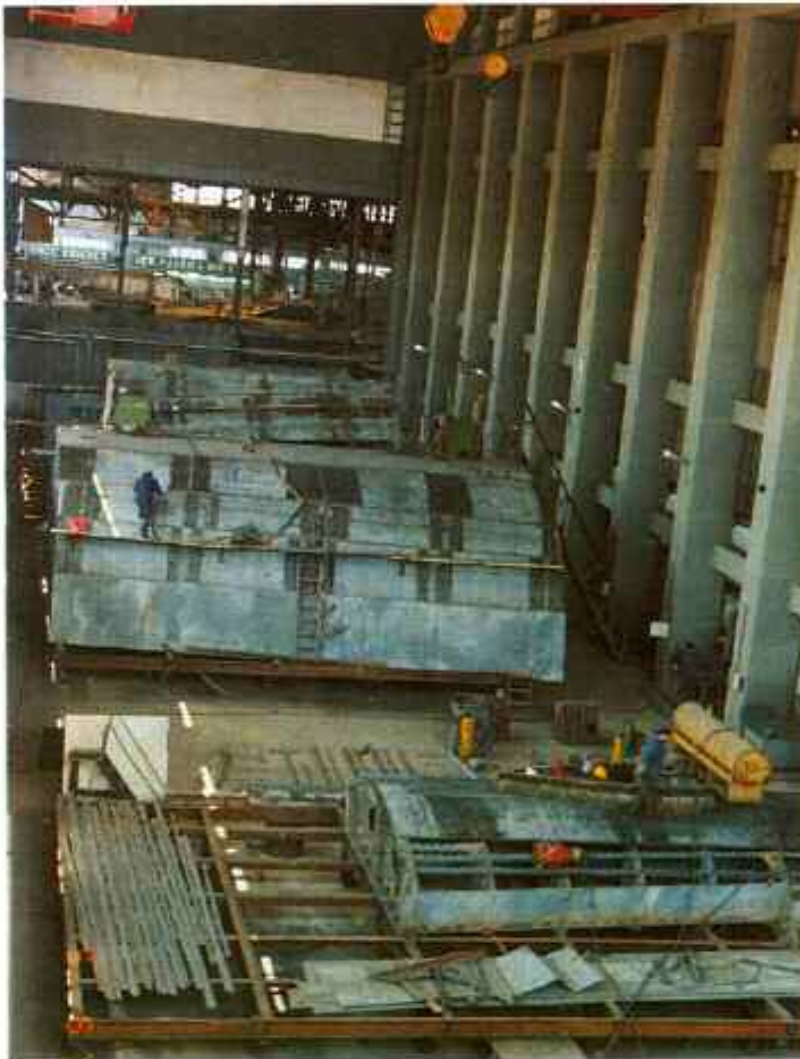
Hull module fabrication in the hull shop.
