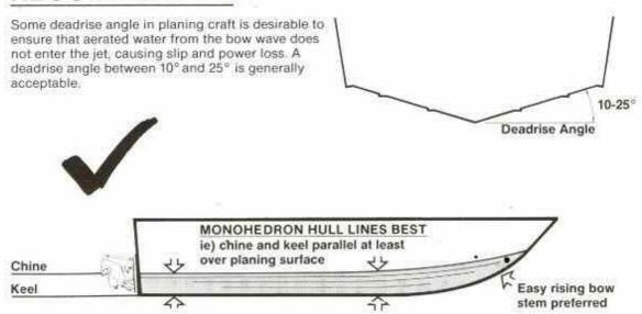
A hull with monohedron lines (ie chine and keel parallel, at least over the planing area) is recommended and gives best handling and performance. An easy rising bow stem is preferable — avoid deep, fine stems, these can cause "bow steer" and ultimately result in poor handling.
