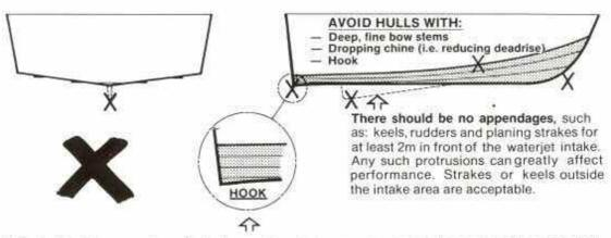
A hooked bottom over the aft planing surface is a common cause of poor handling and high speed broach, it should therefore be avoided.
