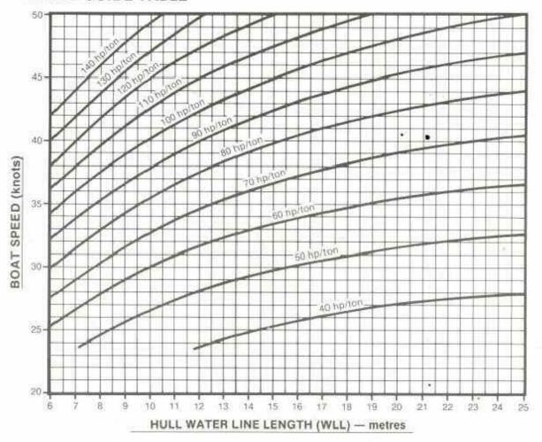
Speeds predicted from this table are approximate only, e.g. deep vee hulls may be 2-3 knots slower. Should an accurate speed estimate be required, hull resistance data can be superimposed over the jet dynamic thrust curves — refer to selected model jet "Designer's Manual".
