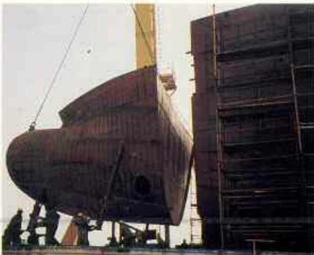
Erection of heavy blocks, performed by 100 t capacity gantry crane.
