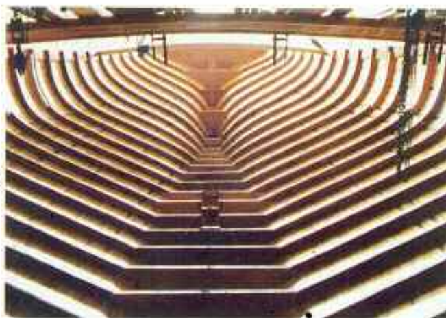
Finished Wood Composite Hull.
