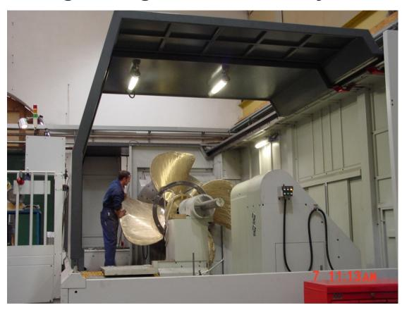
Teignbridge now have a melting capacity of 3 tons. Propellers of up to 2.65 metres in diameter are produced and shafts up to 250mm diameter.
