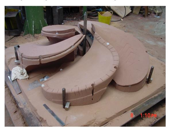
The individual blade moulds are fitted together and the propeller is assembled using a specially adapted base where each blade is slid into place using key ways.
