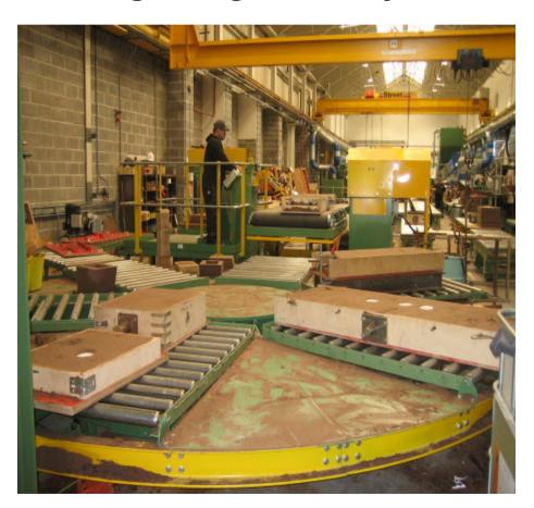
The carousel where moulding of sterngear components and production propellers takes place.
