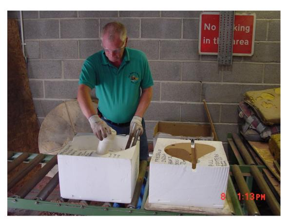
The blocks are filled with sand. Each block makes one half of a blade mould.
