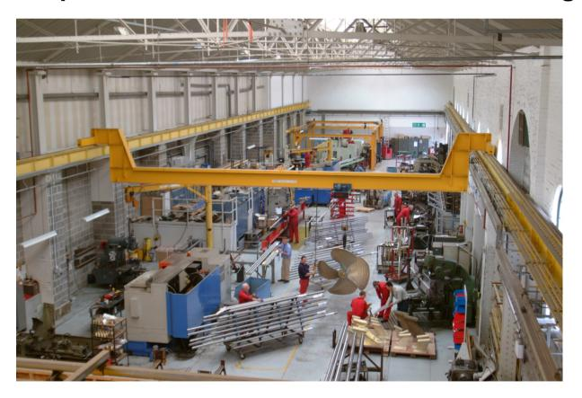
Shafts, P-brackets, rudders and propellers are manufactured in machining cells.
