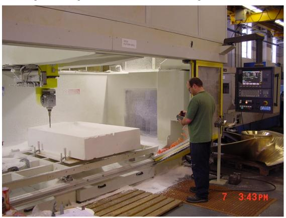
Details of the propeller are downloaded into the 5-axis CNC milling machine which very quickly cuts the blade shape into a high-density polystyrene block. Two blocks are required for each propeller, one for pitch face and one for suction face.
