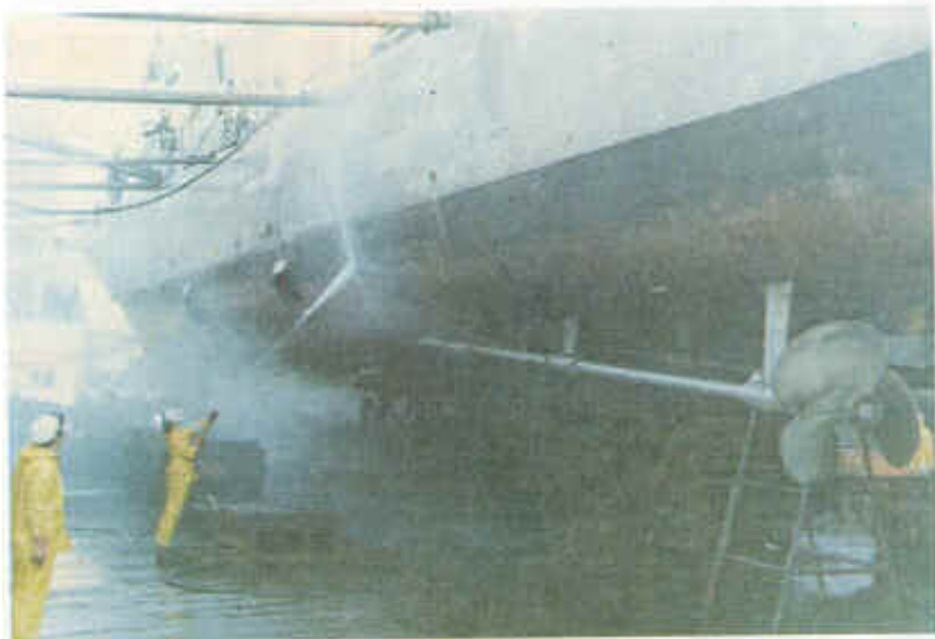
UNDERWATER HULL CLEANING OF A FAST PATROL BOAT BY WATER JET
