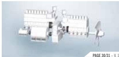
PASSENGER SHIPS THE MULTI-ENGINE, DIESEL-MECHANIC FOUR-STROKE DRIVE
