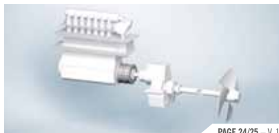
CARGO VESSELS THE TWO-STROKE MAIN PROPULSION DRIVE WITH REDUCTION GEAR
