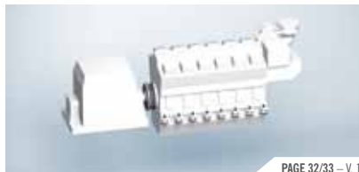
PASSENGER SHIPS THE SEPARATED DIESEL-ELECTRIC DRIVE ARRANGEMENT
