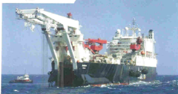
Pipe layer "Solitaire" with LCI propulsion drives 10 x 4.3 MW
