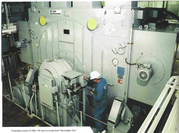
Propulsion motor 15 MW, 135 rpm on cruise liner "Norwegian Sun"
