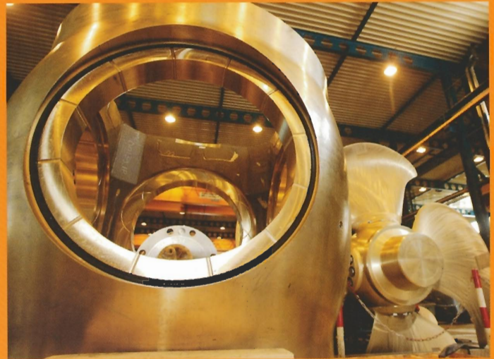
D-hub in machine shop.
